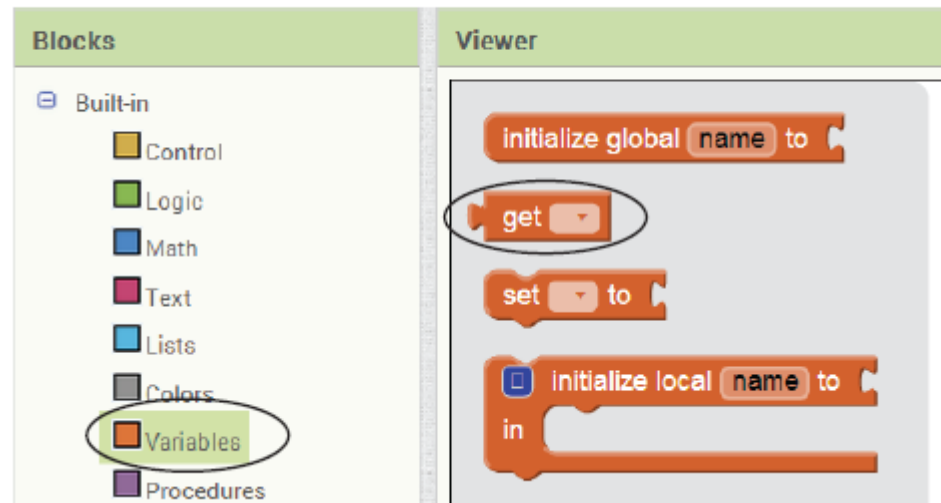
Figure 6-22 Selecting the get Block from the Variables Drawer (Source: MIT App Inventor 2)
