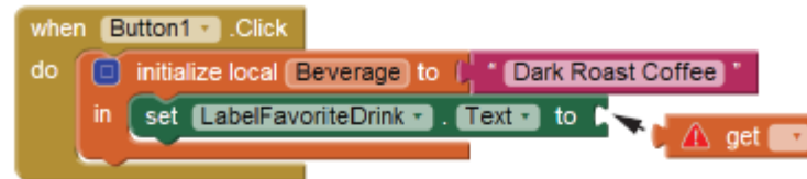
Figure 3-52 Selecting the Beverage Variable for the get Block (Source: MIT App Inventor 2)
