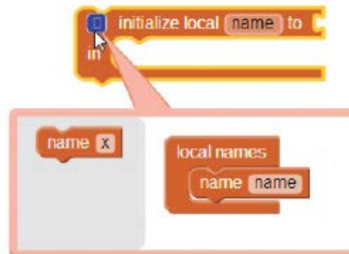
Figure 3-64 Mutator Bubble (Source: MIT App Inventor 2)
