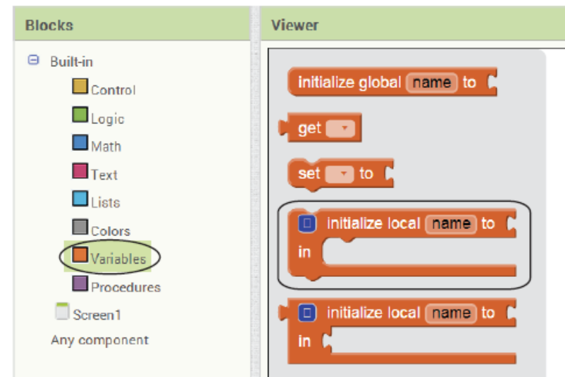
Figure 3-44 Creating a Variable Initialization Block (Source: MIT App Inventor 2)
