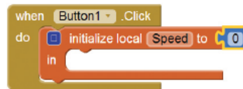
Figure 3-43 Assigning the Number 0 (Source: MIT App Inventor 2)
