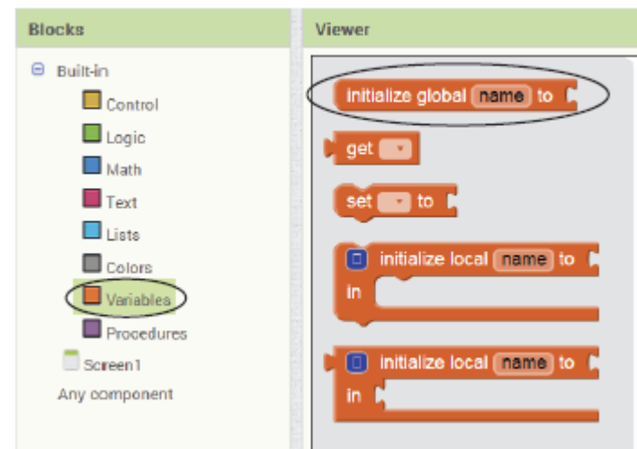
Figure 3-73 Creating a Global Variable Initialization Block (Source: MIT App Inventor 2)
