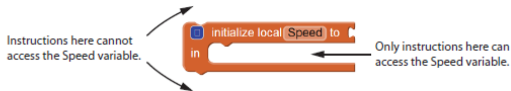
Figure 3-63 The Scope of a Local Variable (Source: MIT App Inventor 2)
