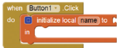
Figure 3-36 An initialize local name to Block Placed Inside a Button's Click Event Handler (Source: MIT App Inventor 2)
