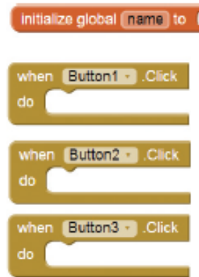
Figure 3-75 Global Variable Initialization Block Outside of All Methods (Source: MIT App Inventor 2)
