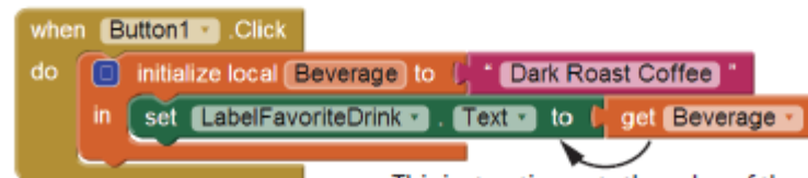
Figure 3-53 The Completed Instruction (Source: MIT App Inventor 2)
