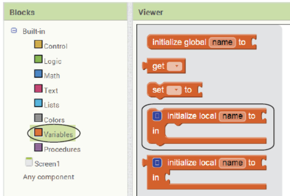
Figure 3-34 Creating a Variable Initialization Block (Source: MIT App Inventor 2)
