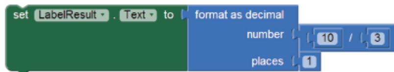
Figure 3-26 Rounding the Result of 10/3 to one decimal place (Source: MIT App Inventor 2)
