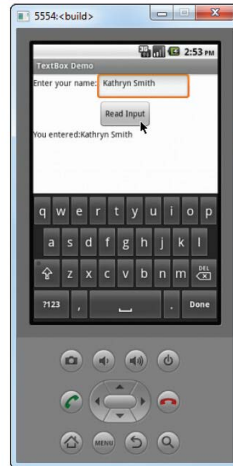
Figure 3-4 The App after the User has Entered Input and Clicked the Button (Source: MIT App Inventor 2)
