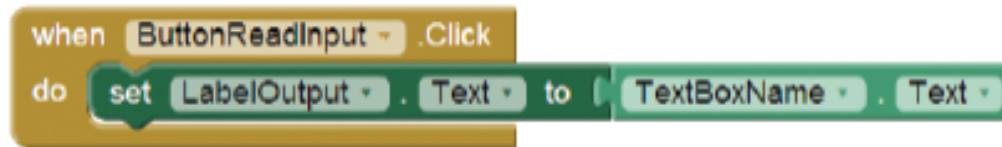
Figure 3-3 The ButtonReadInput Click Event Handler (Source: MIT App Inventor 2)
