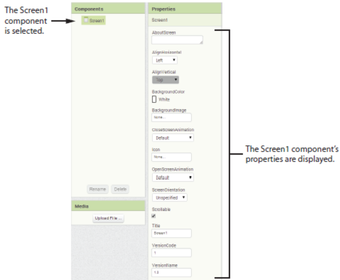
Figure 1-29 The Properties Column, Showing the Selected Component's Properties (Source: MIT App Inventor 2)
